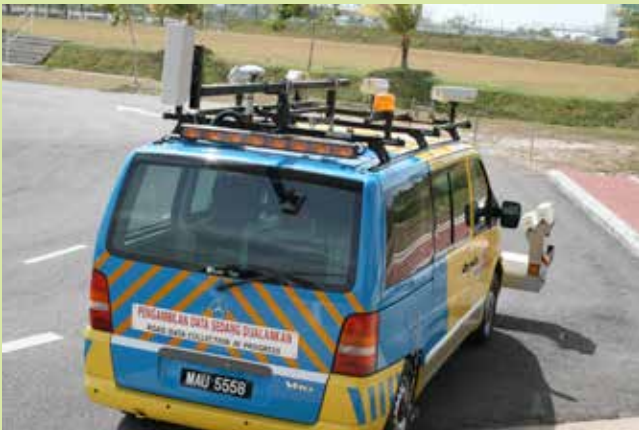
Figure 4 : Asset Camera synchronizing with GPS System
