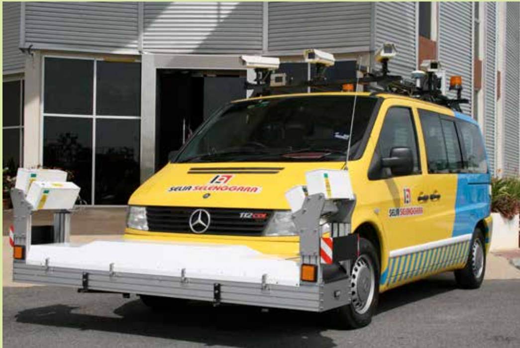
Figure 1 : Integrated Network Survey Vehicle (Selia Scanner)
